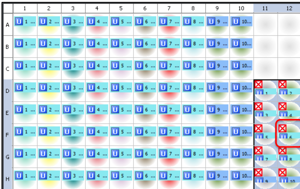
Figure 10: Example plate layout with omitted NTC reactions. The well outlined in red is the NOTCH1 NTC reaction.
